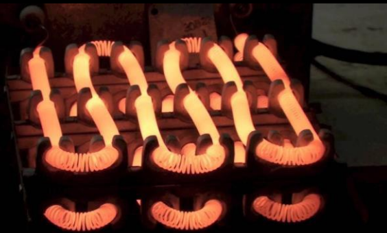
Example of strip heat during operation
